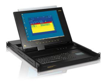
ACS1208AL/ACS1216AL are a LCD KVM Switch at 1U height integrating with a set of 15-inch LCD panel, keyboard and touch panel to save space effectively. Its modularized design facilitates restoration, replacement and maintenance services.
